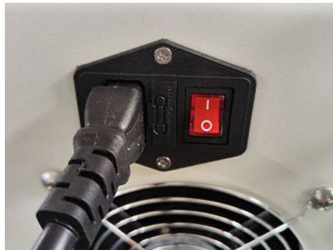
The fuse is located between the socket and the switch.
