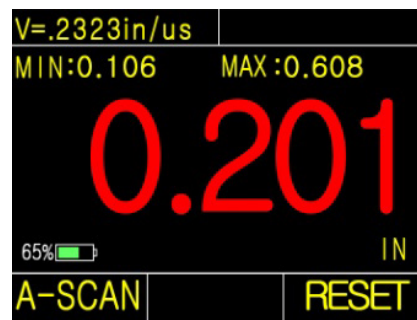
Min / Max Mode, Red Number Indicates Alarm
