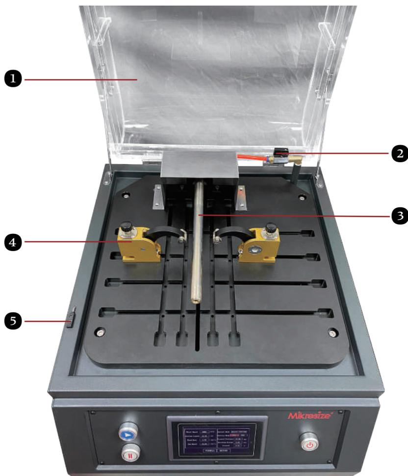
**1. Transparent protective cover: used to prevent cooling water and cutting waste from splashing, and the transparent material makes it easy to observe the state of the cut sample**
