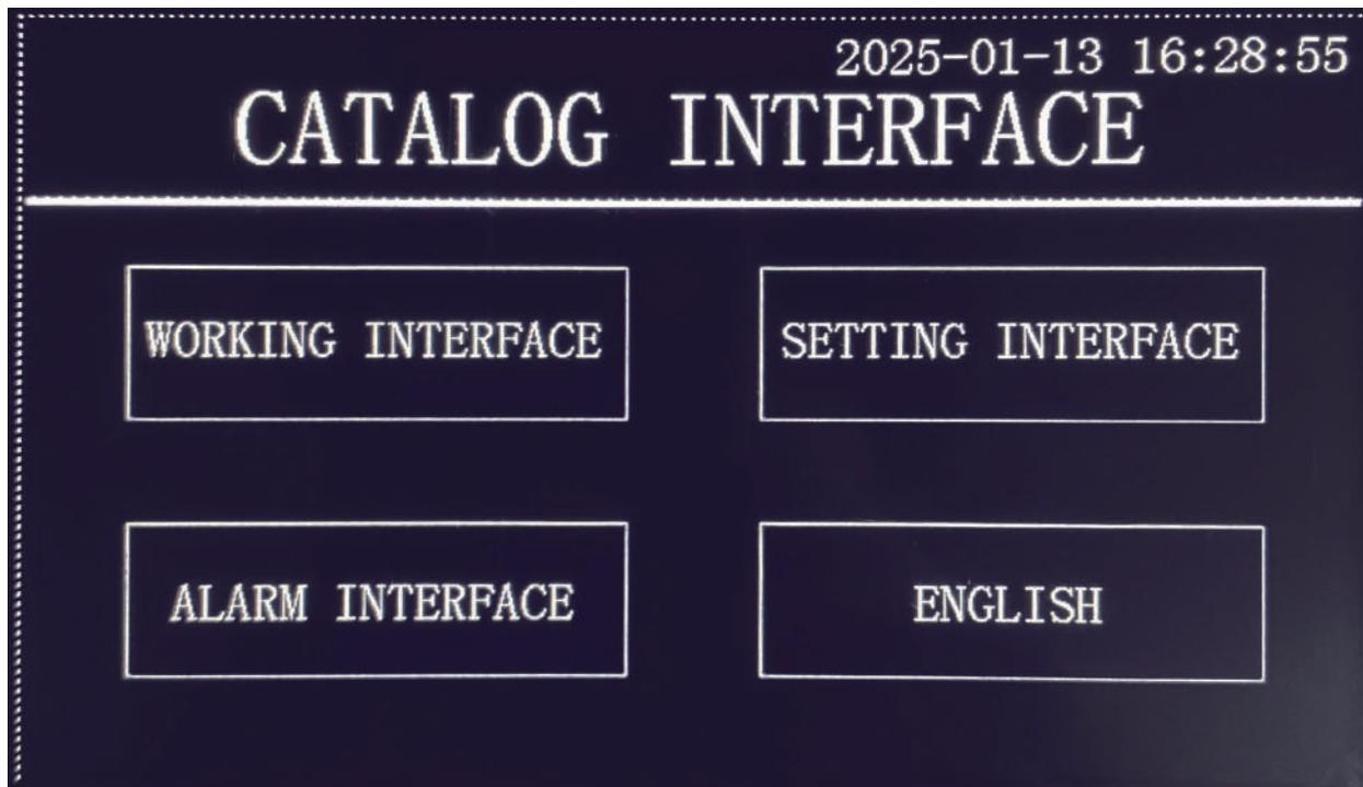
After the device is turned on, it enters the "CATLOG INTERFACE" interface. This device consists of four parts: "WORKING INTERFACE", "SETTING INTERFACE", "ALARM INTERFACE" and "LANGUAGE SWITCHING".
