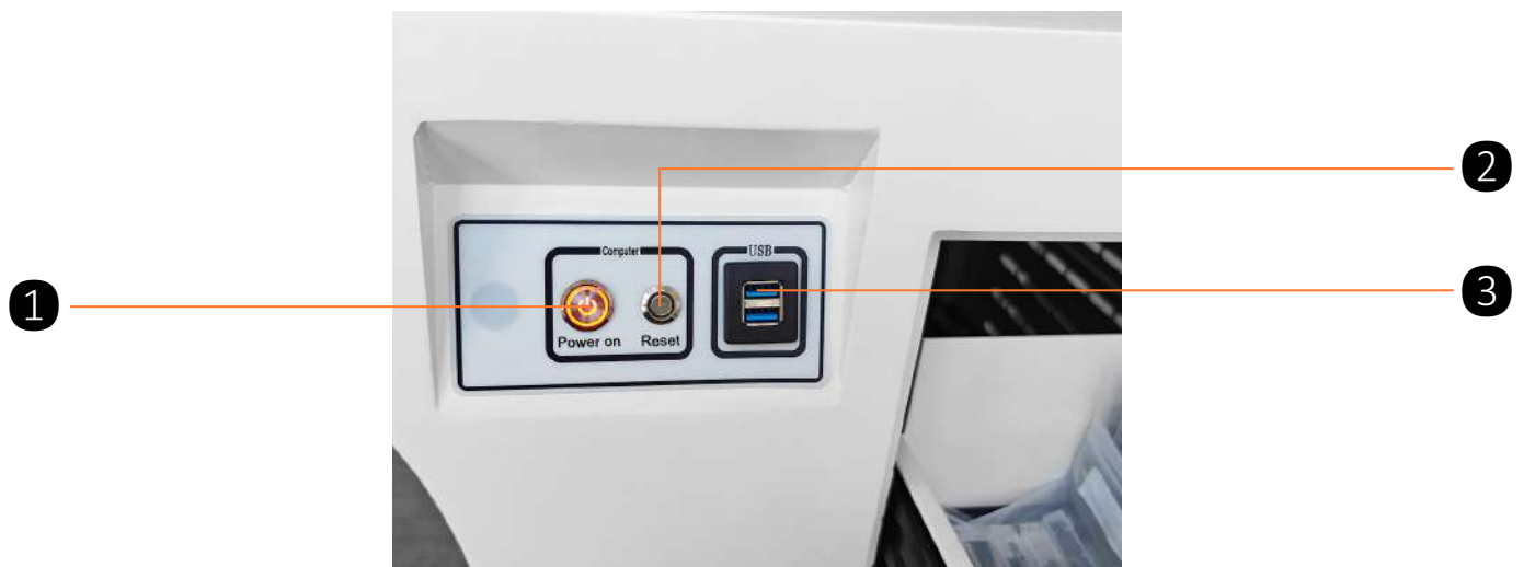
1. Computer Power Button 2. Reset Button 3. Usb Interface
