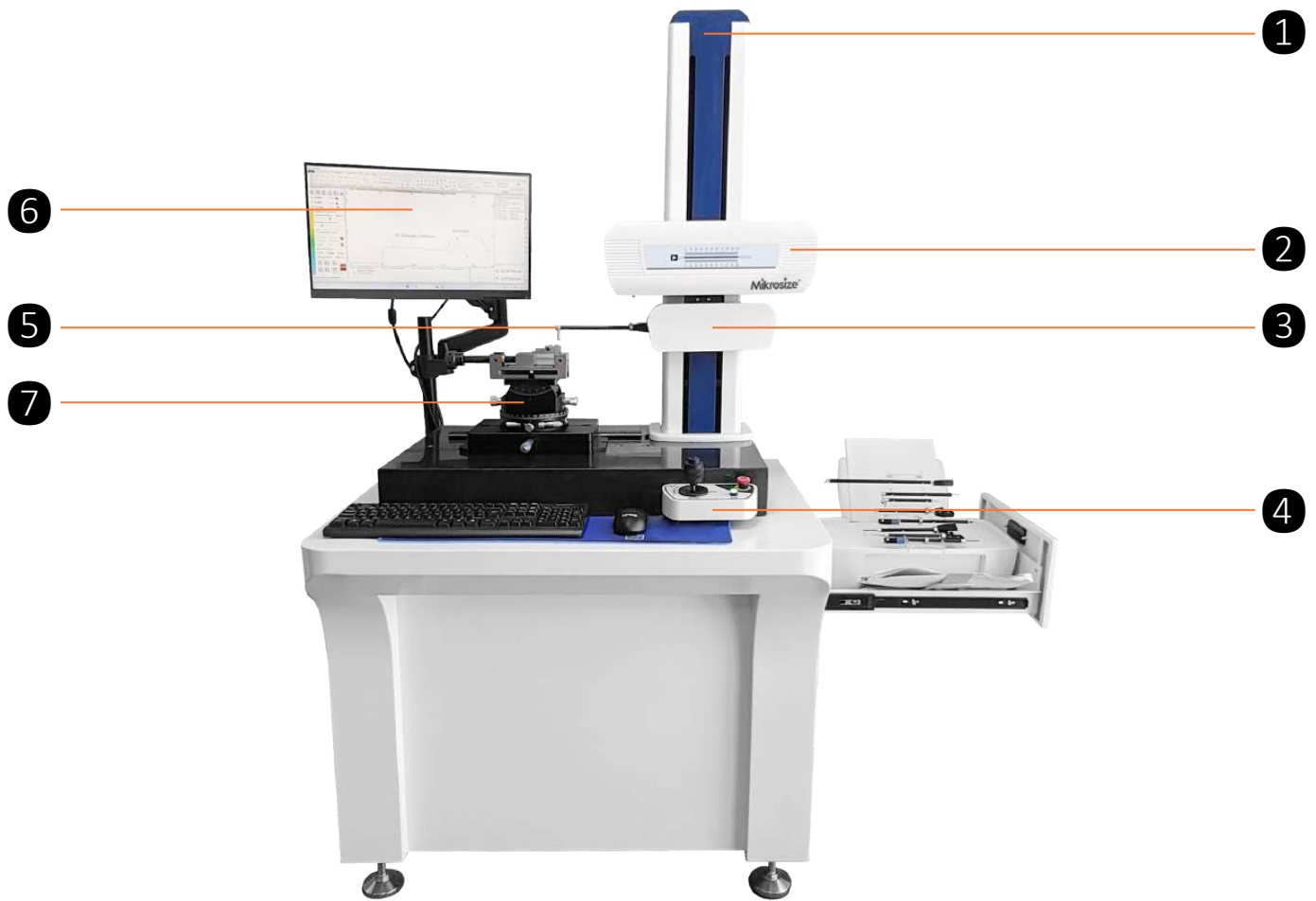
1. Column 2. Horizontal Guideway 3. Grating Sensor 4. Joystick 5. Stylus 6. Display Screen 7. Comprehensive Adjustment Platform
